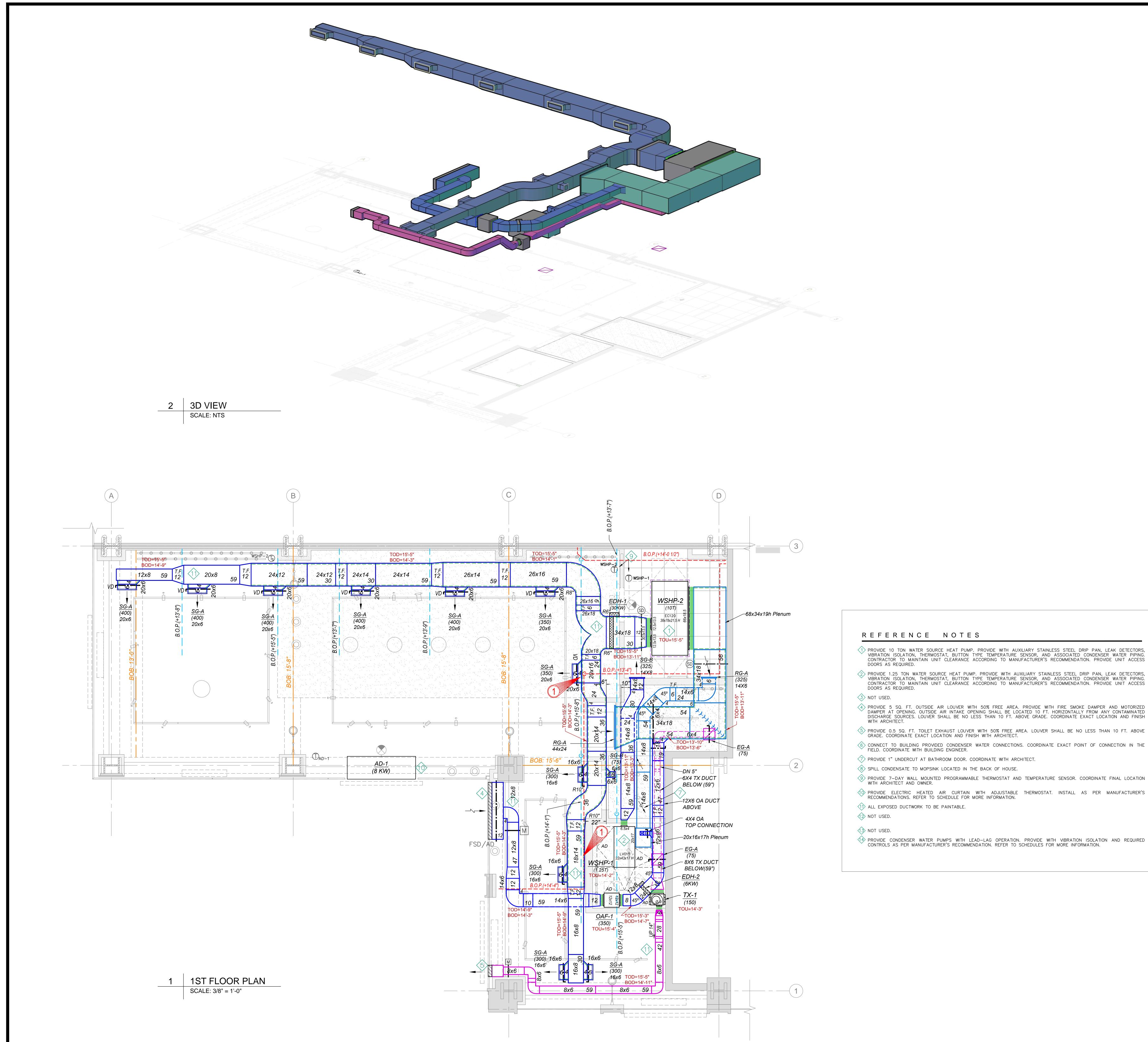
PROVIDE 5 SQ. FT. OUTSIDE AIR LOUVER WITH 50% FREE AREA. PROVIDE WITH FIRE SMOKE DAMPER AND MOTORIZED DAMPER AT OPENING. OUTSIDE AIR INTAKE OPENING SHALL BE LOCATED 10 FT. HORIZONTALLY FROM ANY CONTAMINATED DISCHARGE SOURCES. LOUVER SHALL BE NO LESS THAN 10 FT. ABOVE GRADE. COORDINATE EXACT LOCATION AND FINISH
